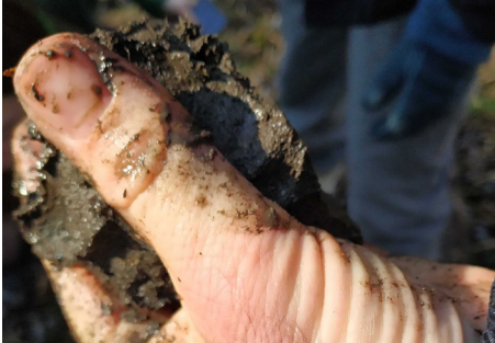
Testing the plasticity of the soil of HOLE
