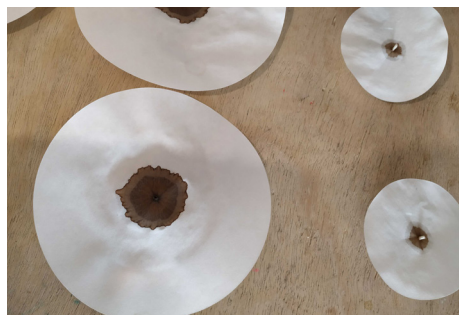
The soil solution penetrates the filter paper
